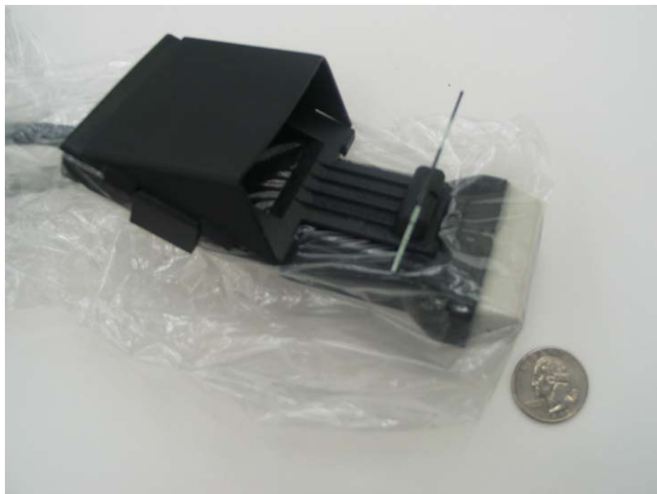
Figure 4. The fully assembled Sonic Flashlight with the plastic probe cover bag enveloping only the base.
