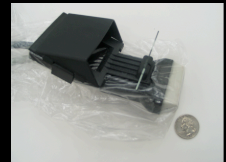
Fig 4. The fully assembled version of the Sonic Flashlight with sterile bag [patent pending]
