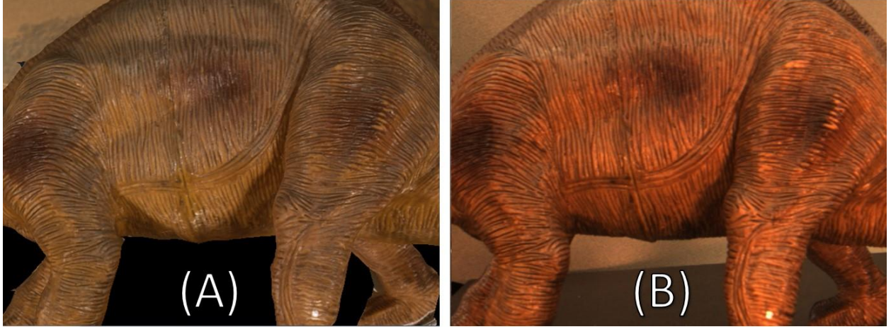
Figure 5-2: Dinosaur model: Pre-acquired surface map (A) , rendered from the correct viewpoint, with the actual camera image (B) (Wang et al. 2014).
