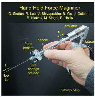
orientations. Preliminary psychophysical evaluation demonstrates that the device improves the ability to detect and differentiate between small forces at the tip of the tool. Magnifying forces in this manner may provide an improved ability to perform delicate surgical procedures, while preserving the flexibility of a hand-held instrument.
