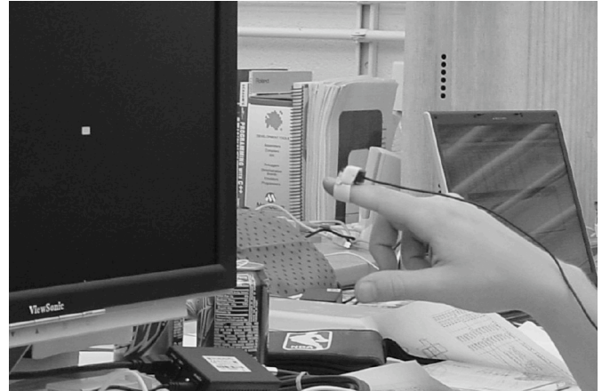
Fig.3. Fingertip-mounted camera controlling the location of a small square target on a screen (miniature vibrator not shown).
