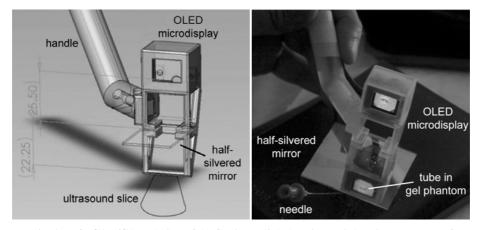
Fig. 1. Left: CAD/CAM design of the Sonic Penlight housing. Right: First prototype of the Sonic Penlight and the insertion of needle into a gel phantom with its guidance.
