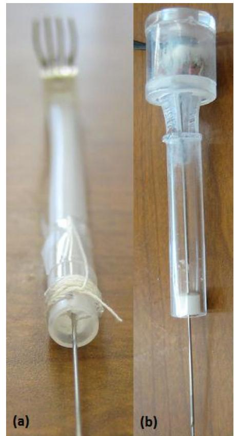
**Figure 4-4.** (a) string guided pressure sensor and (b) needle hub pressure sensor
