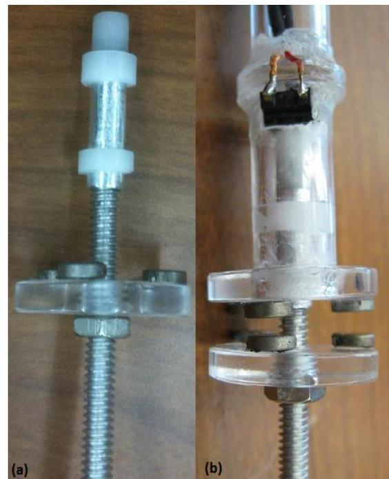
**Figure 4-7.** (a) Threaded rod assembly with Delrin bushings (b) Magnetically stabilized sensor prototype connected to HHFM
