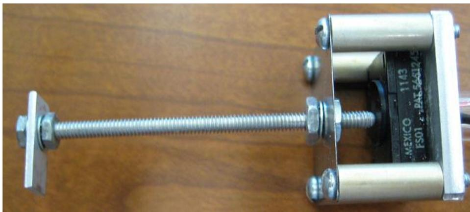
**Figure 4-10.** Shim stock preload prototype.
