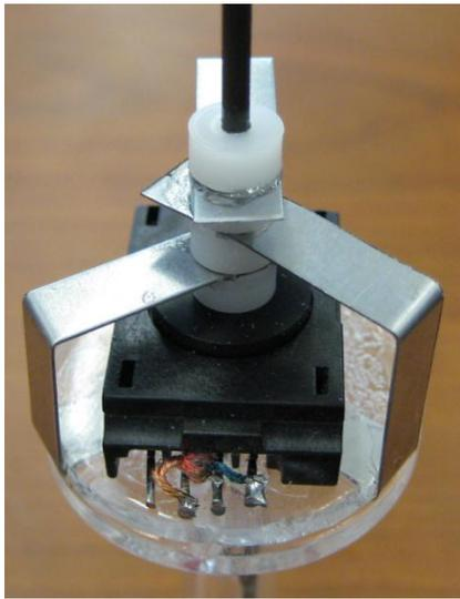
**Figure 4-9.** Leaf spring design in triangular arrangement.
