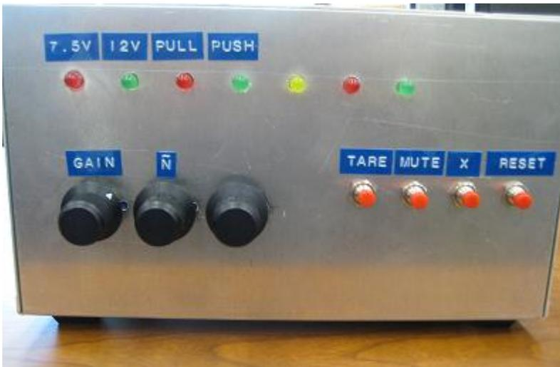
**Figure 4-11.** Front panel to Model-2 electronics enclosure
