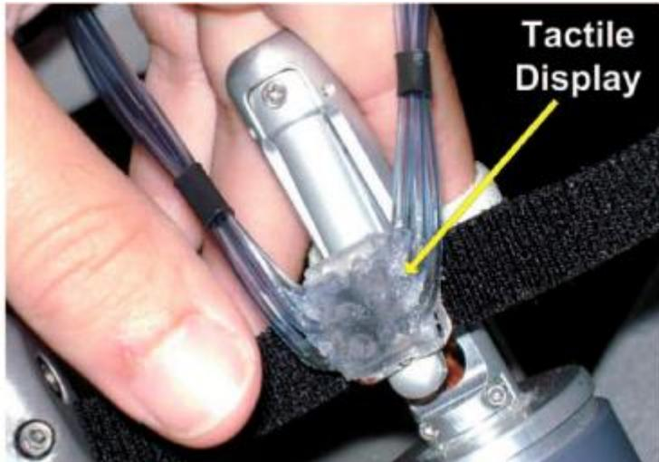
**Figure 2-4.** Tactile display fitted to *da Vinci* control. From [25].
