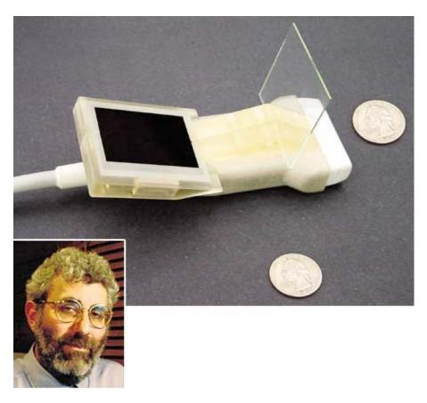
Biomedical engineer George Stetten's Sonic Flashlight [above] lets doctors view ultrasound images directly over the part of a patient's body that's being scanned.
