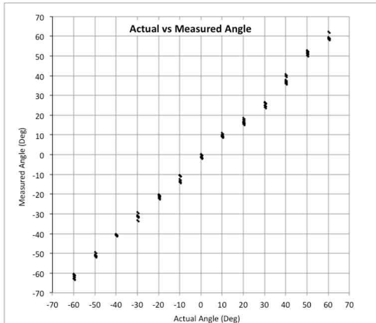
**Fig. 4** Measurements of probe angle relative to the surface of a phantom computed from location of laser spots in video image.
