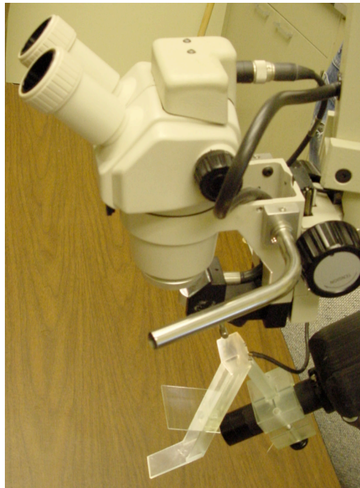
Fig. 6 First-generation OCT penlight positioned under surgical microscope.
