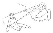
Figure 2. An RTTH display projects a nearly stable virtual image at the actual location of the data in real time, as shown here displaying infrared laser rangefinder data through smoke using an HOE in a fireman's visor.
