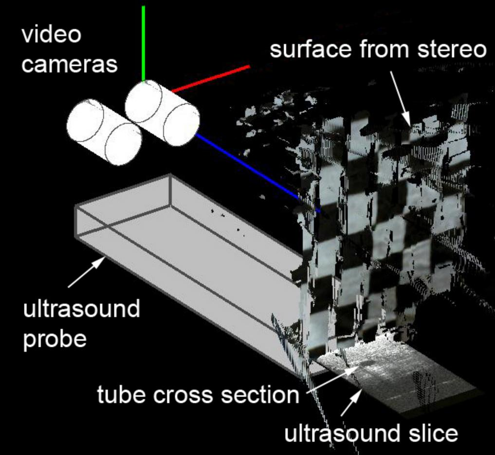
Real-time 3D rendering of the ultrasound probe, the ultrasound data slice, and the surface of the phantom. The ultrasound data and the phantom's surface are correctly positioned relative to one another and to the probe.
