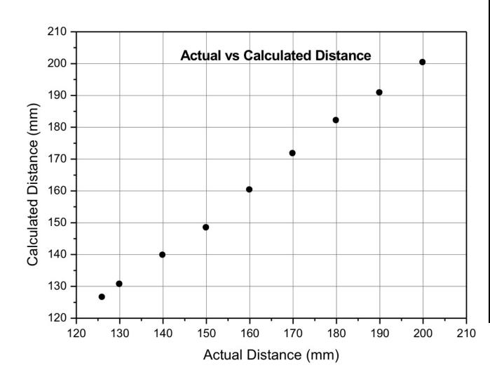
The RMS error in our system's distance measurements is ±1 mm.
