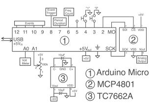
The new system, which we call the "Micro-BLIP", appears to a host computer via USB as a human typing on a standard computer keyboard. Thus, the data from the Micro-BLIP will be entered into any word processor or spreadsheet program. No special software is required on the host computer, which can be based on any standard operating system.
