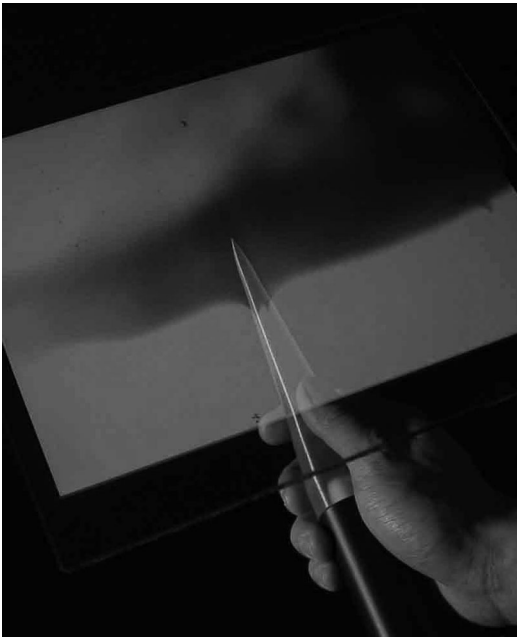
Fig. 9. View through the mirror of the apparatus depicted in Fig. 8. The master controller is a mockup of a micropipette. Although not an actual master-slave system in this example, moving the target (fish egg) into the actual slave effector (micropipette) gives the illusion of piercing the egg with the hand-held device.
