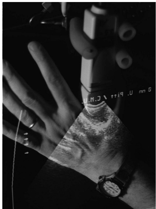
Fig. 3. Photograph, from the viewpoint of the operator, showing a scan of a hand using the apparatus in Fig. 2. The reflected ultrasound image is merged with the direct visual image.
