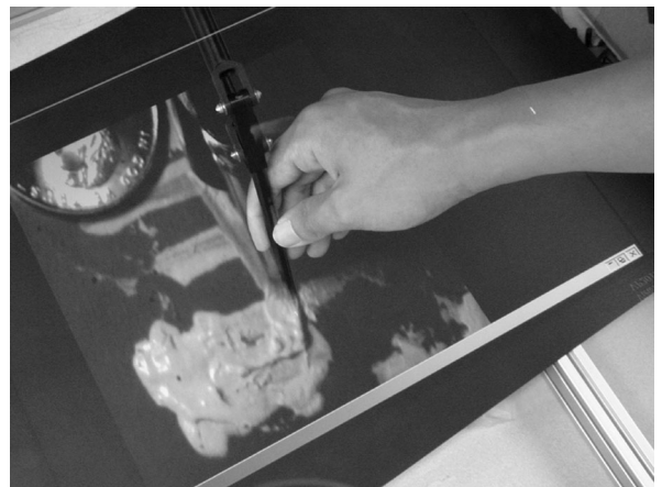
Fig. 13. The Micropainter system as viewed through the half-silvered mirror by the operator, showing the master handle registered with the remote paintbrush and paint. The remote environment is 10 times as small (notice the scale of the penny). Author David Wang is painting his name in Chinese.
