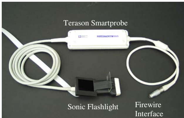
Figure 2. The Sonic Flashlight built around the Terason Smartprobe ultrasound machine, using a 10MHz linear probe. The ultrasound machine interfaces with a laptop computer via an IEEE 1394 Firewire interface.
