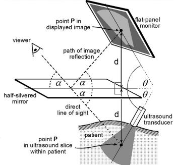
**Figure 2.** Geometric relationships for the Sonic Flashlight. The mirror bisects the angle between the display and the virtual image. By fundamental laws of optics, the virtual image will appear at its physical location, independent of viewer position.
