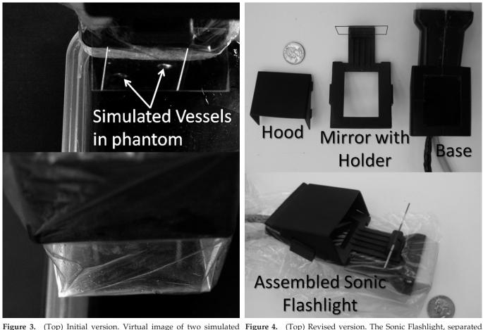
vessels in a phantom seen through the half-silvered mirror with the into three pieces, from left to right: hood, mirror with holder, and plastic probe cover over the base only. (Bottom) The same virtual base. (Bottom) The assembled Sonic Flashlight with the plastic image seen through the half-silvered mirror with the plastic probe probe cover enveloping only the base. cover over the mirror. Note the degradation of image quality.
