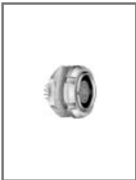
ECG.2G Fixed receptacle with two nuts, key (G), straight contact for printed circuit (back panel mounting)
