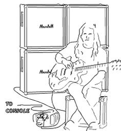
The most widespread use of DI boxes is with guitar pick-ups or keyboards. The optimal setting for this is most likely with the pad switch set to 0dB, although with some high-output pick-ups the performance of the AR-133 may be improved if the pad switch is set to 20dB to prevent possible clipping of the input. The instrument is connected to the 1/4" jack socket, and a parallel feed taken from the other jack socket to the instruments' own amplifier.
