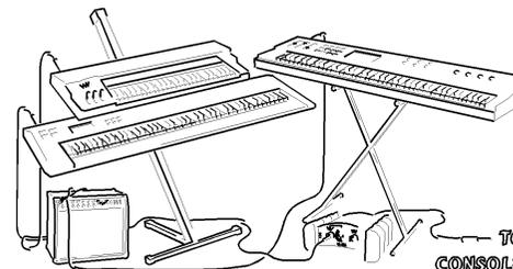
Where 2 or 3 keyboards are used by a single performer, it is possible to reduce the number of DI's needed if a mixer/amplifier is used by the performer for his or her personal monitoring. A single AR-133 can be fed either from a line-level output from the head (pad set to 20dB) or from the amplifier power output (speaker output) (pad set to 40dB).
