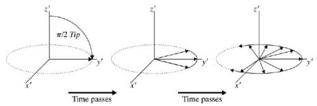
A. T2-weighted images are primarily dependent upon this mechanism to generate contrast between tissues.
