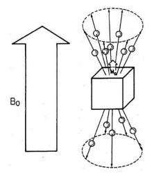
A. The net magnetization at rest  $\mathbf{M}_0$  within a voxel is aligned with the magnetic field  $\mathbf{B}_0$  produced by the superconducting magnet.
