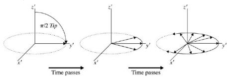
**A.** The rate at which the components de-phase is a function solely of the local chemical environment, and is not effected by  $\mathbf{B}_0$  field inhomogeneity.
