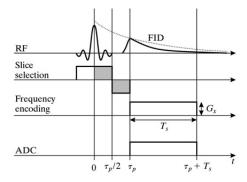
**A.** A short  $\mathbf{B}_1$  field containing a band of frequencies used to tip the longitudinal magnetization into the transverse plane.
