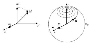
A.  $B_1$  is the magnetic field created by the RF coils to tip the longitudinal magnetization into the transverse plane.
