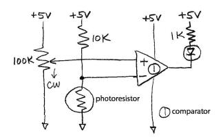
A. Turning the potentiometer clockwise (CW) will raise the voltage on the (+) input of the comparator.
