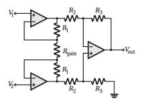
A. It shows a differential amplifier, also known as an "instrumentation" amplifier.
