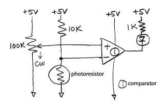
**A.** Although the comparator may be an open-collector device, the circuit can still function since the LED is tied to +5V by the 1K resistor.
