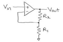
A. This is a non-inverting amplifier circuit.
