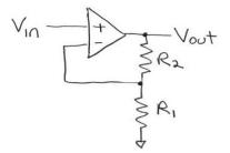
A. Vout will not change, no matter how much current a load may draw from the output of the circuit.
