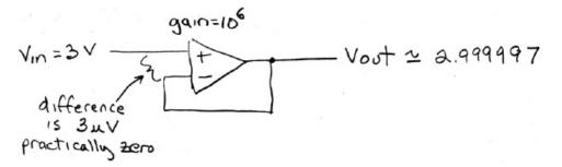
**A.** It shows how the voltage between the inputs of a real op amp with feedback is not actually zero, but rather very small.
