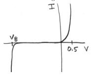
**A.** When the component is back-biased, the current is in the opposite direction from the voltage.
