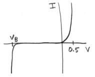
A. It represents the current as a function of voltage for a diode.
