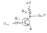
A. Ignoring the base-emitter voltage drop, the base current  $I_B$  will be 1 mA.
