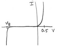
A.  $V_B$  is the "base" voltage of the forward biased base-emitter junction, for the transistor within the diode.
