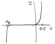
**A.** As in the relationship between current and voltage for all passive components, the curve passes through the origin.
