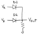
**A.** With actual diodes,  $V_{out}$  will always be a little bit (~ 0.5V) below both  $V_A$  and  $V_B$ .
