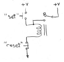
A. The "reset" switch is a momentary pushbutton that is normally open (NO).
