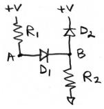
**A.** The voltage at node B is 3.0 V.
